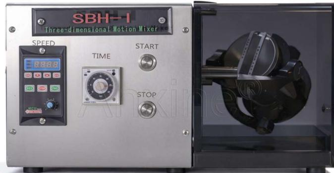
The SBH-I Micro Three-Dimensional Mixer is designed for mixing freely flowing powder or granular materials to achieve a high level of uniformity among substances with different physical properties. It is also capable of mixing various liquids. This model is especially suitable for laboratory use. Its application fields include the pharmaceutical, chemical, food, electronic technology, sintered metal, ceramic, and cosmetics industries.
