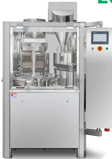
As a high-output automatic capsule filler, the NJP-2000C fills up to 150,000 capsules per hour. It works with capsule sizes 00# to 4#. This machine fills powders, granules, and pellets into different types of capsules. It supports stable operation, automatic capsule rejection, and easy cleaning without removing molds. This automatic filling model is for large-scale pharmaceutical production, offering quality and efficiency for capsule packaging.
