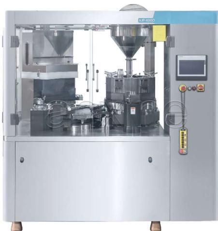
The NJP-4000D is a fully automatic capsule filling machine. It is used for large-scale pharmaceutical and supplement production, ideal for both powder and pellet filling. The machine handles a wide range of capsule sizes (from 00# to 5#) with consistent dosing precision. Its production is up to 4,000 capsules per minute.
