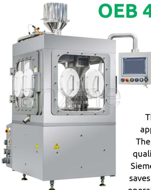
The NJP-703 OEB 4 Ultra is an advanced automatic capsule filling machine. It is designed for high-containment production of potent drugs. It also strictly meets OEB 4 safety standards. It offers precise dosing with a high-precision metering disc. The machine fully automates capsule sorting, filling, and closing. It supports capsule sizes from 00# to 5# and fills up to 42,000 capsules per hour.
