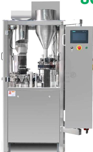
The NJP-800C is a reliable machine that fills empty capsules with medicine powder, tiny pellets, or granules. It finishes the whole production process by itself. This capsule filler picks up empty capsules, opens and fills them with the right amount of powder. Then it closes the capsules perfectly. This model works fast, filling up to 48,000 capsules every hour.
