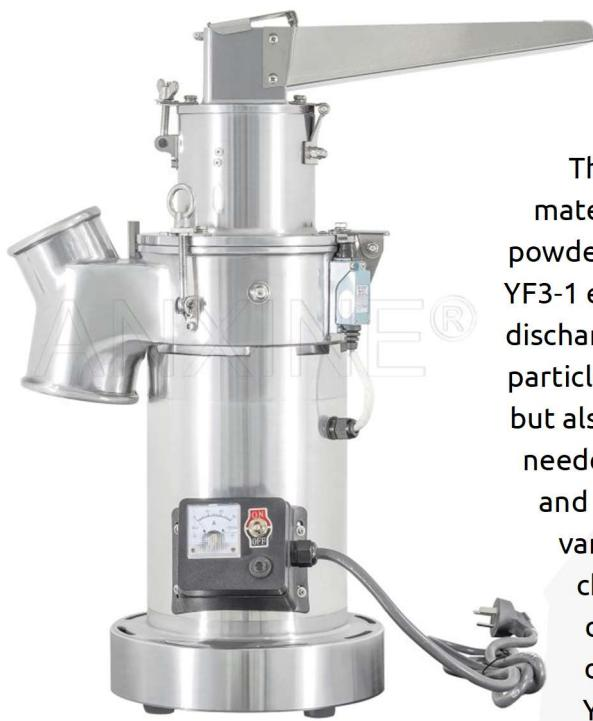
The YF3-1 airflow superfine pulverizer is a compact and powerful machine. It is designed for the precision grinding of dry materials of different types. It is widely used in the pharmaceutical, food, chemical industries, and research labs.
