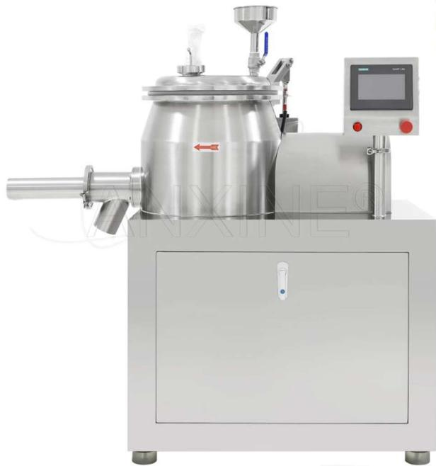
At the core of the CHL Series is its advanced high-shear mixing and granulation mechanism. The design integrates a rotating impeller for intense mixing of dry powders with liquid binders, creating homogeneous wet masses that are then processed into uniform granules via a secondary chopper. Constructed with food-grade 304/316L stainless steel, the CHL Series features
