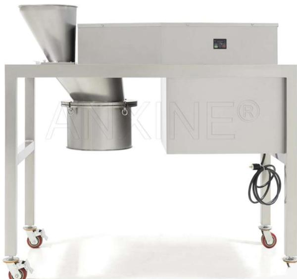
The CFZ Series are multi-purpose machines designed to crush, granulate, and refine materials into uniform particles. They are applied to both dry and wet materials. The CFZ machines are especially suited for processing materials like dried herbs, chili powders, rice powders, tablets for regranulation, food powders, and agricultural products. They are widely used in the pharmaceutical, food, and chemical industries for breaking lumps.
