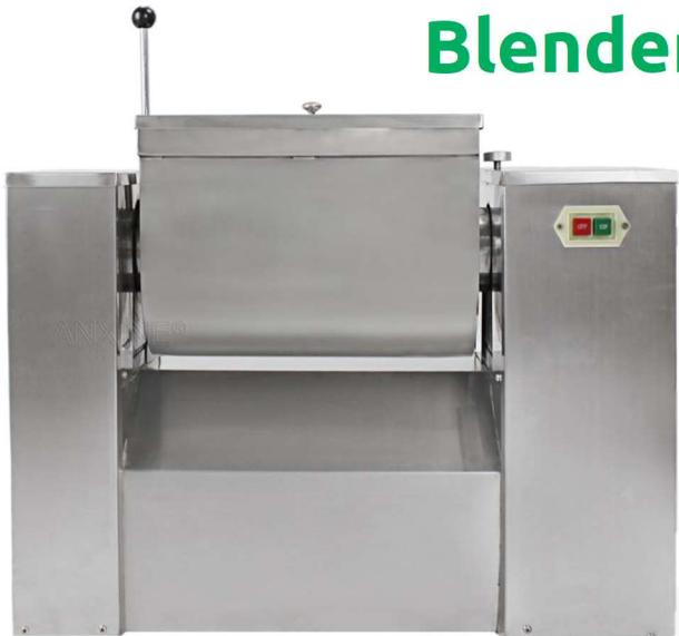
The CH-series trough mixers, including CH10 and CH20, belong to the horizontal mixer. They are designed for gentle and efficient blending of dry powders and granules, ideal for precise powder blending. With 10L and 20L capacities, they are well-suited for lab-scale production or small-batch formulations. They are useful in industries such as pharmaceuticals and R&D.
