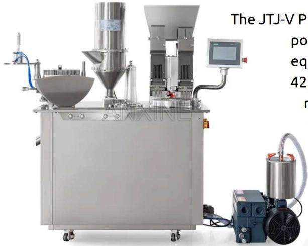
The JTJ-V Pro+ is designed for small to medium batch production. It fills powder or tiny granules into different types of capsules. The equipment handles capsule sizes from 00# to 4# and fills up to 42,000 capsules per hour. It features PLC control, variable speed motors, and an easy-to-clean design. This capsule filler suits pharmaceutical, health supplement, and lab-scale production.
