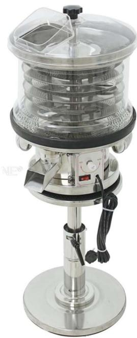
As The ATD-310 Rotary Vibration Dust Remover makes sure your tablets are spotless, even for large batches. It uses unique rotary vibration to gently remove all dust and tiny bits from the tablet surface. This important step means your tablets stay perfect, and your equipment will last longer. With the ATD-310, you get consistently clean tablets, a faster production flow, and full compliance with GMP standards.
