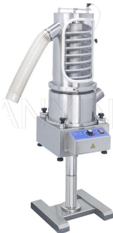
The ATU-750 is a machine that cleans and elevates tablets at the same time. It gently removes dust and small imperfections while moving the tablets upwards. Its unique "uphill" motion saves space. It prevents re-contamination or damage that can happen with other transfer systems. You will continue to receive high-quality tablets delivered directly to the next machine.
