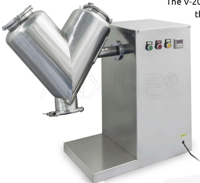
The V-20 Mixer is designed to blend dry powders and granules in the pharmaceutical, chemical, and food industries. Its simple structure and compact size make it ideal for small-scale production and laboratory use. The V-20 uses a V-shaped mixing barrel for even distribution of materials.
