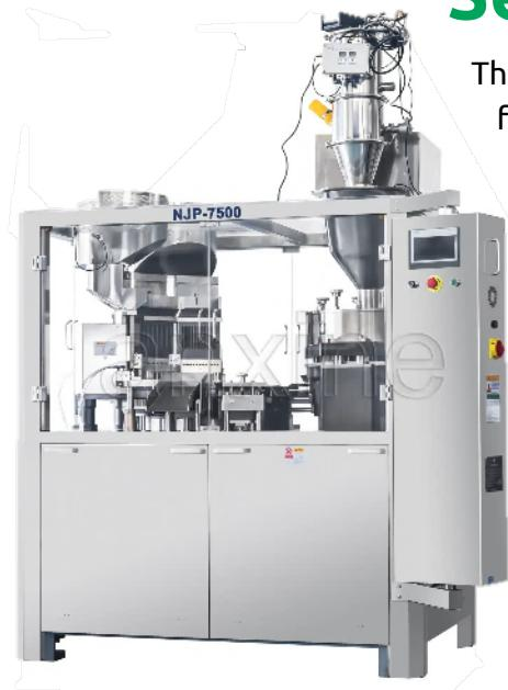
The NJP-C Series is a comprehensive lineup of fully automatic capsule filling equipment engineered to cover all production demands, from small-scale batches to large-volume manufacturing. With maximum outputs ranging from 24,000 to 450,000 capsules per hour, the series offers exceptional versatility—supporting capsule sizes from 0#-4# up to 00#-5# (including safety capsules for select models) and accommodating powders, granules, and pellets.
