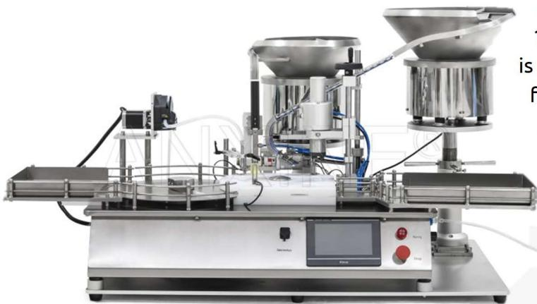
The ceramic pump handles thick or thin liquids without contamination. The adjustable capping head ensures tight seals every time. Safety features like an emergency stop button and grounded power protect users for safe operation. Whether you're bottling serums, supplements, or samples, this machine delivers fast and consistent results.
