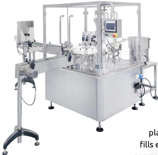
The CGS-1 automatic model is made for filling and capping small dropper bottles. It can fill liquids like eye drops, oils, or other products. It uses a peristaltic pump, which gently moves the liquid through a soft tube and into the bottle. The machine picks up each cap and tightens it automatically. Sensors check for missing bottles or caps so nothing is wasted. The whole system is clean, safe, and easy to use. It's a good fit for small bottle production in medicine, skincare, or lab use.
