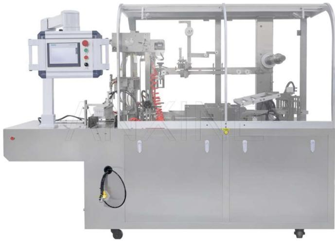
This cellophane wrapping machine offers a fast, automated solution for wrapping boxed items using clear film. It's compatible with cellophane and other packaging materials like OPP, BOPP, and PVC. The TMP-400S is great for gift sets, media boxes, healthcare items, and more. Looking to wrap both single and multi-box packs? This overwrapper got you covered.
