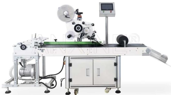
The T-11500 automatic card labeling machine is a high-performance labeling solution developed specifically for all types of cards and flat products.
