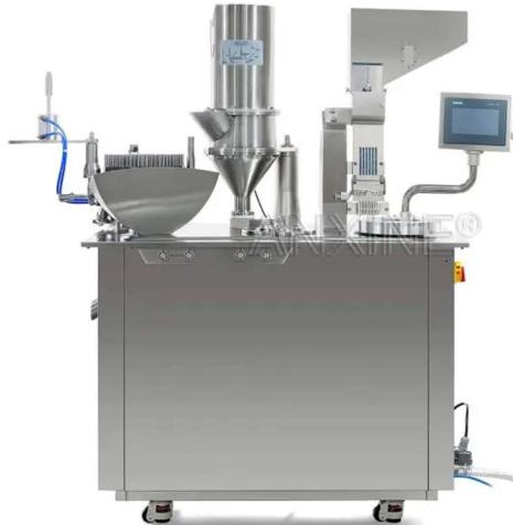
The JTJ-V model produces up to 25,000 capsules per hour. It supports capsule sizes ranging from 00# to 4#, making it suitable for filling powders, pellets, and granules. The machine uses a vacuum system to separate capsule bodies and caps. Then it fills and locks them in place with a mold-based mechanism.
