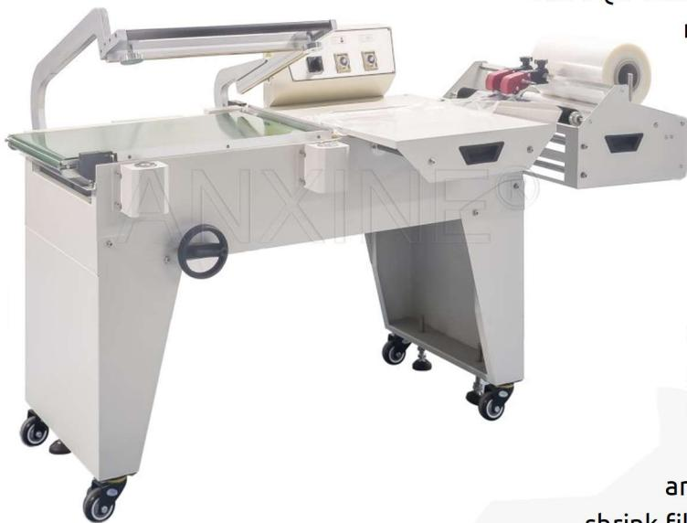
The FQL-450A is a semi-automatic L-bar sealer machine, which means you need a skilled operator to use the equipment. This model is engineered for fast sealing and trimming plastic film before shrink application. With its quick-action sealing arm and overload protection, the FQL-450A offers a smooth solution for clean-cut packaging prep.
