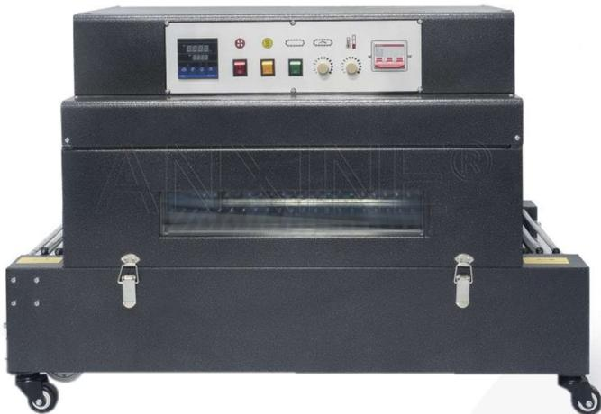
This is a compact, reliable heat shrink tunnel with conveyor. Made for food, pharmaceuticals, and daily-use products, this model uses advanced heat pipe tech and an infrared shrink tunnel chamber to provide consistent shrinking. The DS-H400 also features a stepless speed regulator and a smart temperature controller that adapts to different packaging materials for best results.
