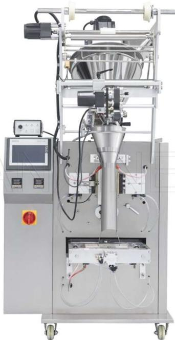
The DXD-300F automatic powder packing machine is a high-tech solution for efficiently and precisely packaging powder. It automatically measures, fills, and seals, so every bag has the same product. This machine can handle different types of powders. These include medicines and food additives. It reliably processes all of them. It uses the latest technology for fast, accurate operations and strict quality control, making it ideal for modern production needs.
